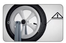
Align the front tire between the front fork ensuring that the tire rotation direction matches the rear tire and directional arrow on the tire. The recommended / maximum tire inflation pressure is **2,5 bar**. DO NOT OVER-INFLATE!
