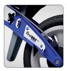
Apply adhesive stickers (Part G) according to the included Sticker Position photos. Note that the adhesive sticker for handlebar should be placed over the plastic cover (Part C).
