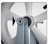
Insert the self-locking nut (Part F) into the hexagonal hole on the left side of the fork and insert and tighten the wheel bolt (Part E) from the right side using the hexagon ("Allen") wrench (Part G).
