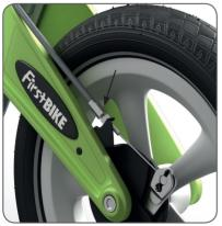
If necessary, adjust the brake cable tension with the adjustment screw located at the end of the brake cable by the rear wheel to ensure the brake does not rub or engage when the brake is not applied.
