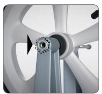
Insert the self-locking nut (Part E) into the hexagonal hole on the left side of the fork and insert and tighten the wheel bolt (Part D) from the right side using the hexagon ("Allen") wrench (Part F).
