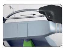
The distance between the handlebar and the brake lever can be adjusted by tightening or loosening the brake lever screw.
